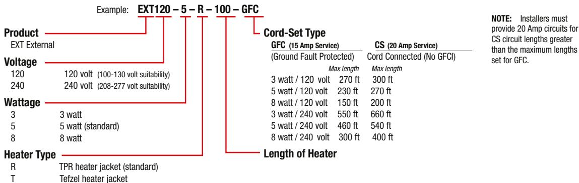
**NOTE:** Installers must provide 20 Amp circuits for CS circuit lengths greater than the maximum lengths set for GFC.
